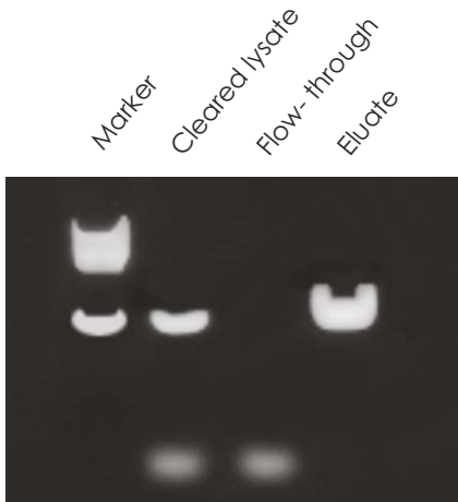
Agarose Gel Analysis showing a step by step pDNA isolation using mdi Express 96 pDNA Miniprep Kit.
